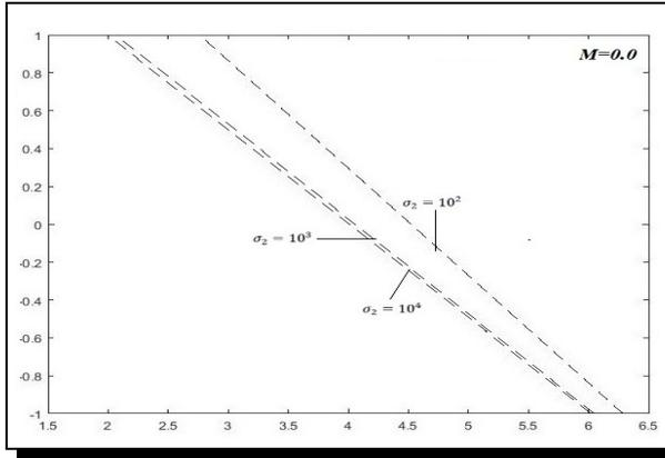
**Figure 4.** Axial velocity,  $u(\xi)$  for  $\bar{\alpha} = 0.1$  and  $\sigma_1 = 10^1$  and  $M = 0$
