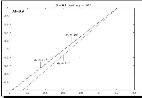
**Figure 8.** Axial velocity,  $u(\xi)$  for  $\bar{\alpha} = 0.1$  and  $\sigma_2 = 10^1$  and  $M = 0$
