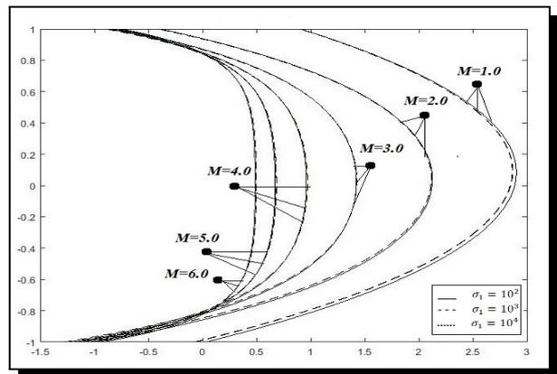
**Figure 7.** Axial velocity,  $u(\xi)$  for  $\bar{\alpha} = 0.5$  and  $\sigma_2 = 10^1$  and different values of  $M$
