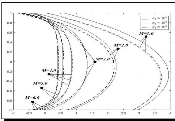
**Figure 2.** Axial velocity,  $u(\xi)$  for  $\bar{\alpha} = 0.1$  and  $\sigma_1 = 10^1$  and different values of  $M$
