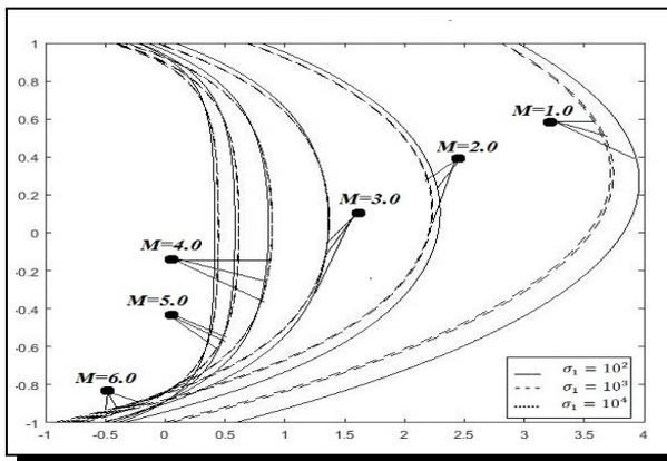
**Figure 6.** Axial velocity,  $u(\xi)$  for  $\bar{\alpha} = 0.1$  and  $\sigma_2 = 10^1$  and different values of  $M$
