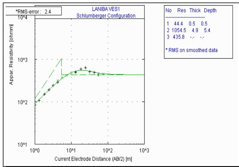
Figure 2. A typical K curve type
