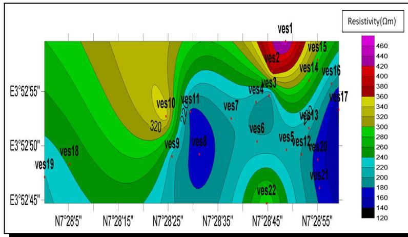
Figure 7d. Iso-resistivity at 75 m depth
