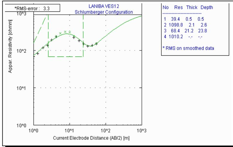
Figure 3. A typical KH curve type
