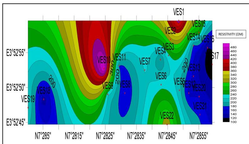
Figure 7c. Iso-resistivity at 55 m depth
