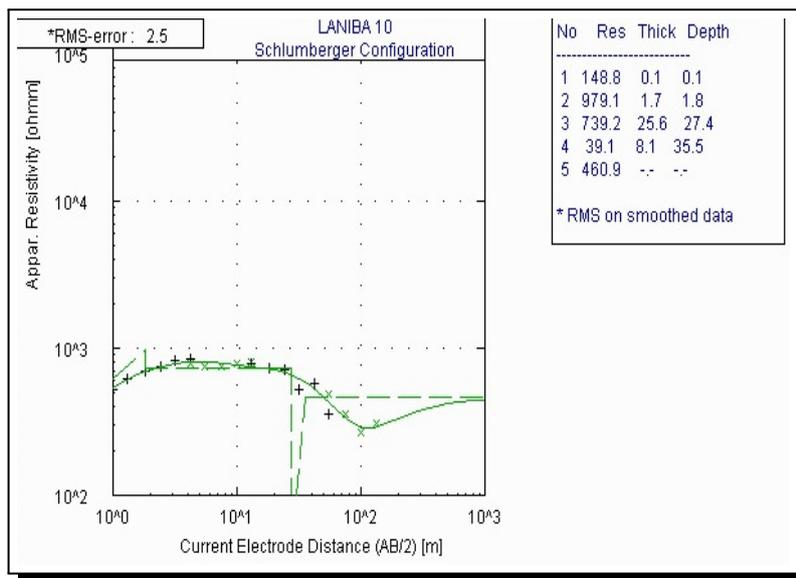
Figure 6. A typical HKH curve type
