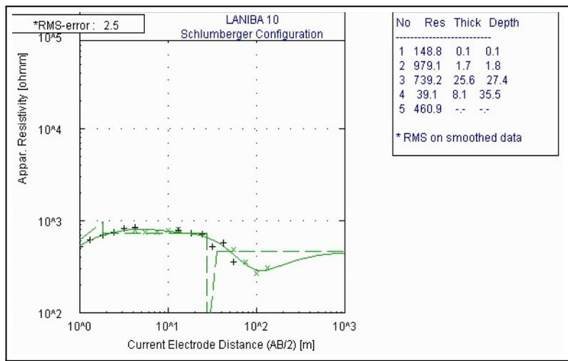
Figure 5. A typical KQH curve type
