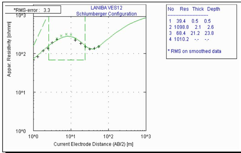
Figure 4. A typical AK curve type
