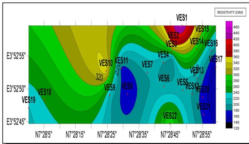
Figure 7b. Iso-resistivity at 13 m depth
