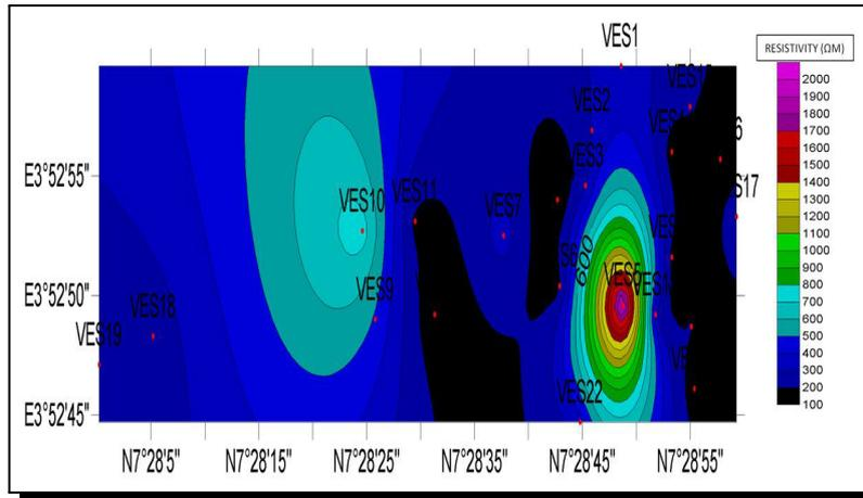
Figure 7a. Iso-resistivity at 5.5 m depth
