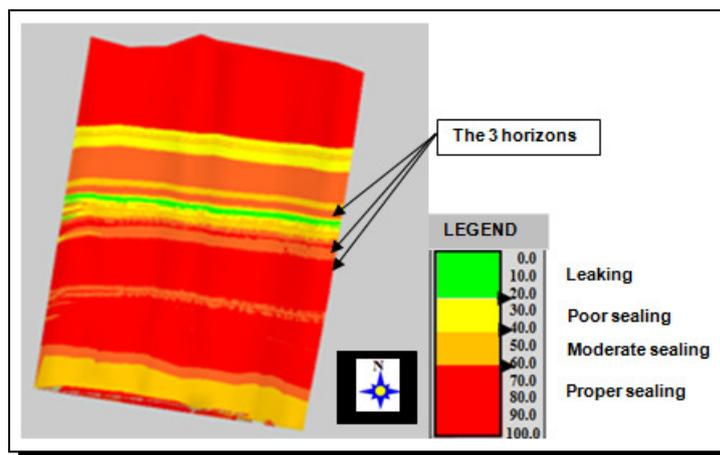
**Figure 11.** Shale gouge ratio of the “Covenant” field
