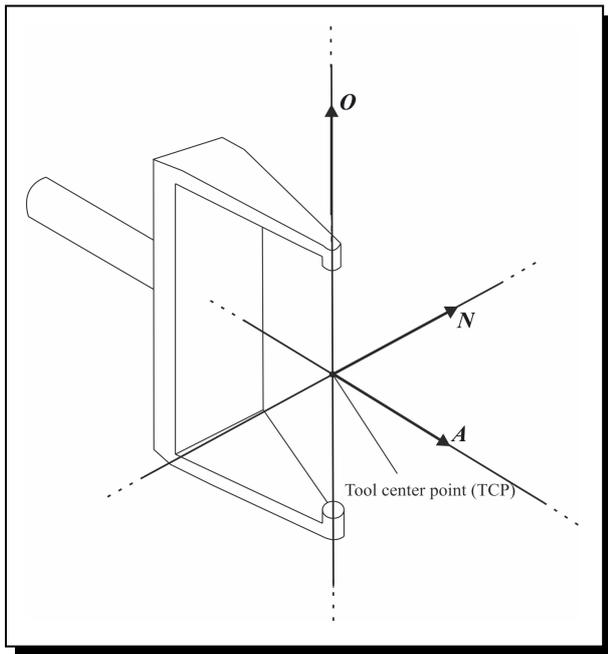
Figure 4. Dual tool frame of a robot end-effector.
