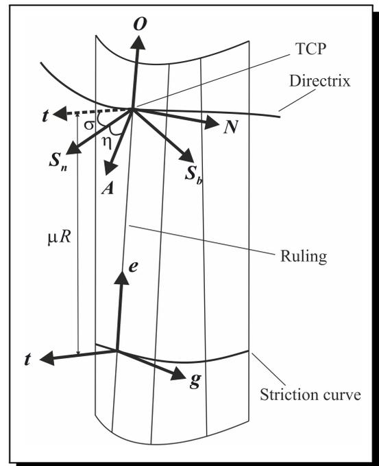
**Figure 3.** Relations between three reference frames as a robot end-effector moves on a specified trajectory.
