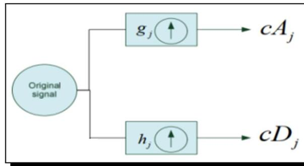
**Figure 2.** The DWT and SWT in one-level of decomposition
