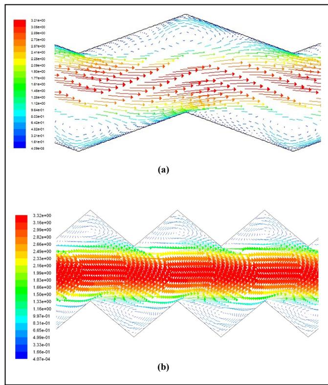
**Figure 6.** Contours velocity vector for  $Re = 1400$  (a)  $\alpha = 20^\circ$  (b)  $\alpha = 40^\circ$
