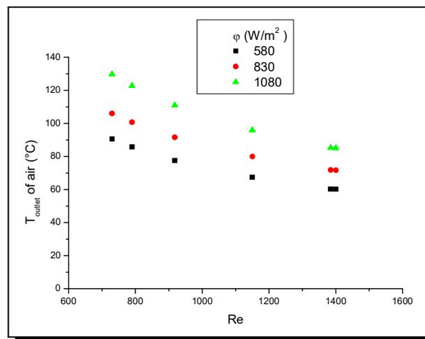
**Figure 12.** Variation of the outlet air temperature versus Reynolds number for different heat flux
