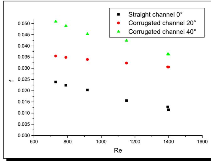
Figure 7. Effect of corrugation angles on friction coefficient
