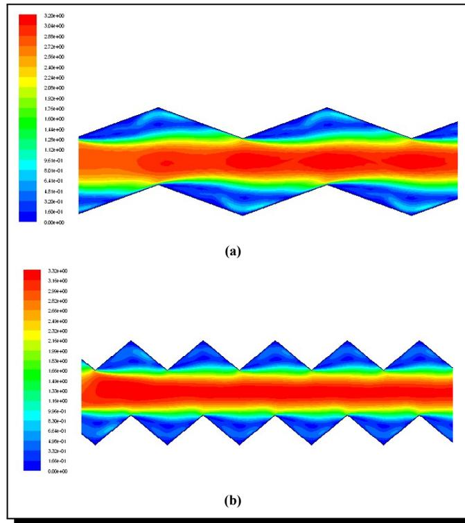
**Figure 5.** Contours of the average velocity for  $Re = 1400$  (a)  $\alpha = 20^\circ$  (b)  $\alpha = 40^\circ$
