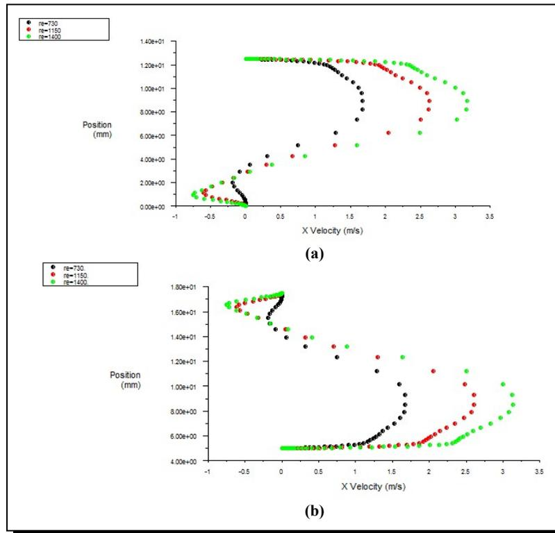
**Figure 3.** Profiles of the horizontal velocity with  $h/w = 0.458$  for different Reynolds (a)  $x = 81.81 \text{ mm}$  (b)  $x = 95.445 \text{ mm}$
