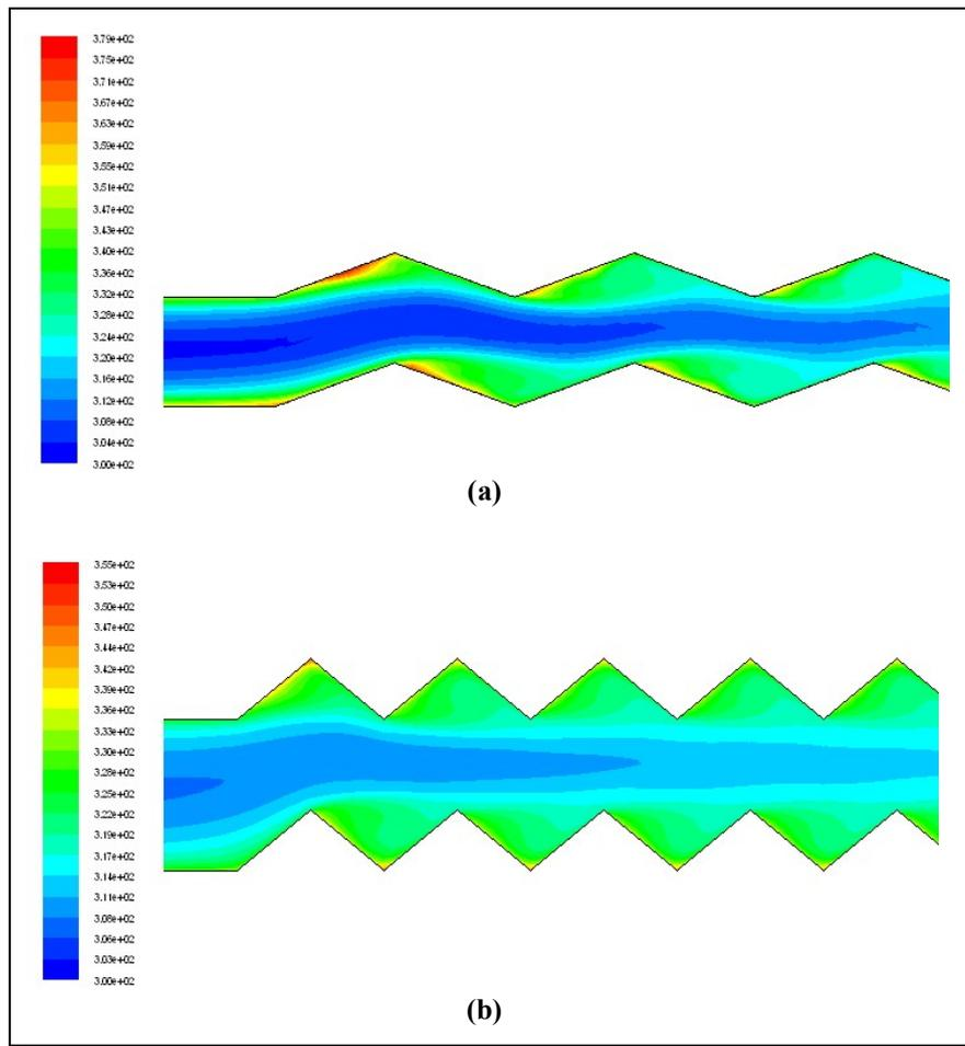
Figure 8. Contours of static temperature for  $Re = 1400$  (a)  $\alpha = 20^\circ$  (b)  $\alpha = 40^\circ$
