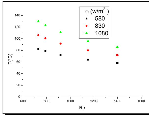
**Figure 11.** Variation of average surface plate temperature versus Reynolds number for different heat flux
