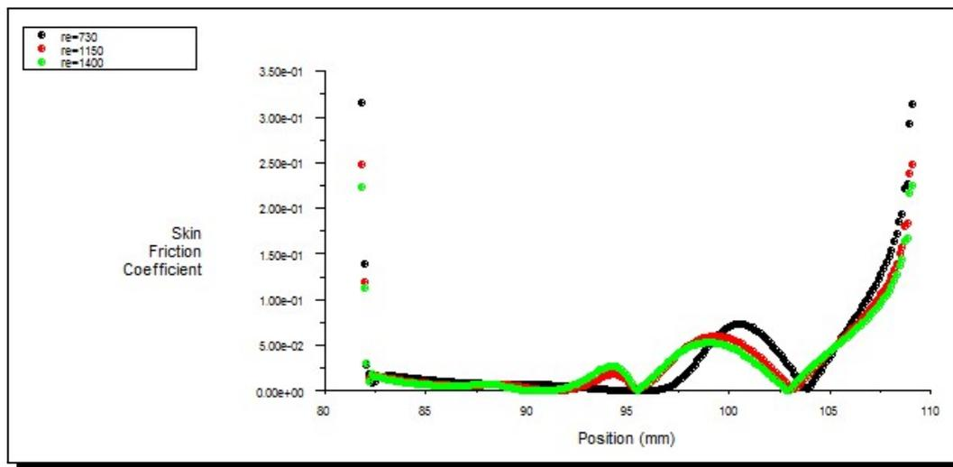
**Figure 4.** Distribution of the local friction coefficient for different Reynolds number with  $h/w = 0.458$  for periodic corrugation (upper wall)
