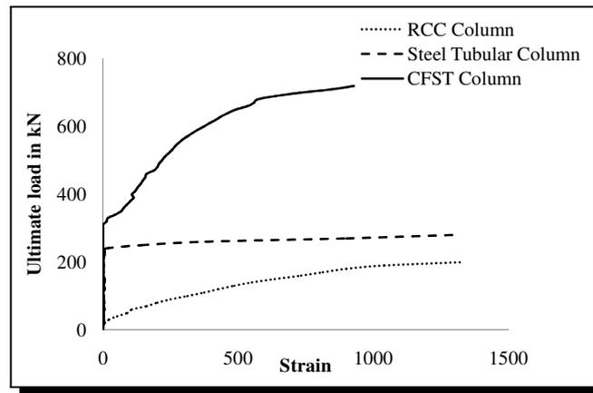
Figure 8. Load-Strain behaviour of the HST, RCC and CFST columns
