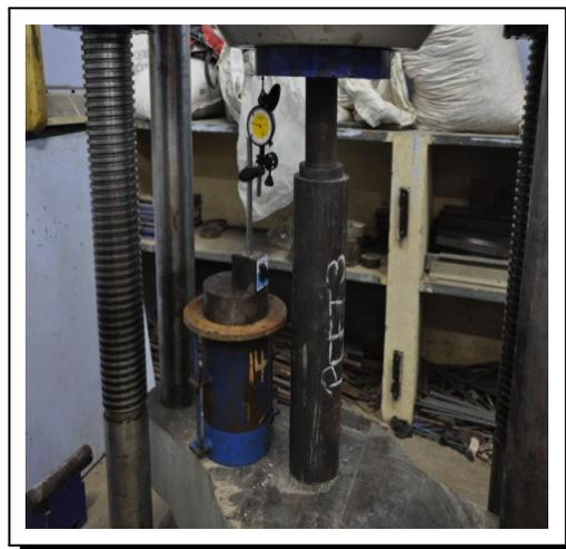
Figure 3. Push out test of the specimen
