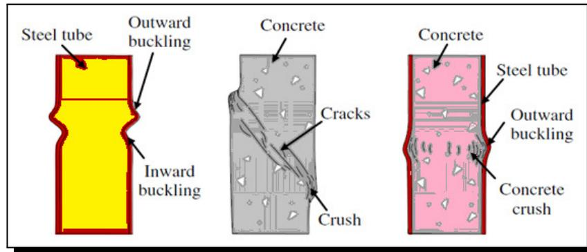
**Figure 6.** Schematic failure modes of the HST, RCC and CFST columns
