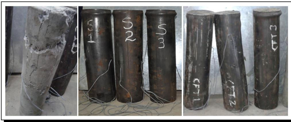
Figure 2. Specimens after buckling
