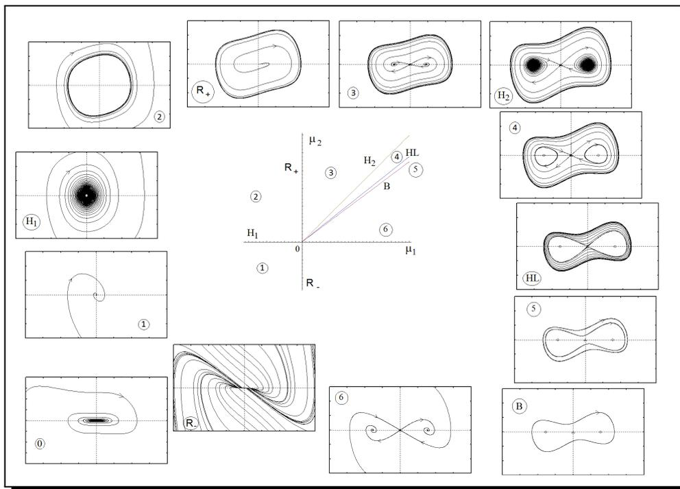
Figure 1. The bifurcation diagram for the double-zero bifurcation, case  $\sigma = -1$ .
